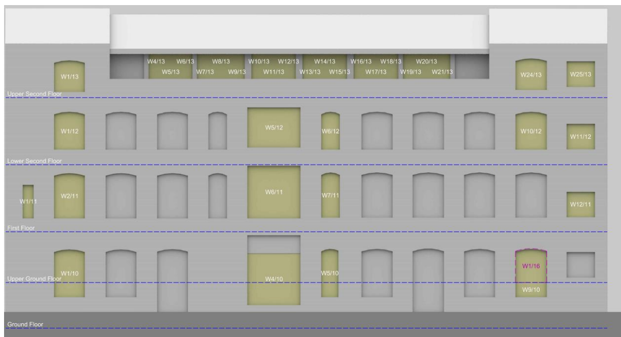
Image 38 – Windows tested at The Ironworks
